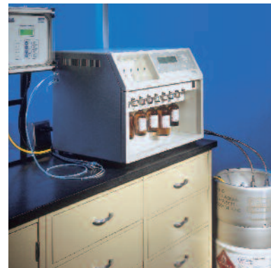
Sealed solvent dispensing directly into DNA synthesizers maintains the lowest possible water content. Solvent levels are monitored by an electronic level sensor.
