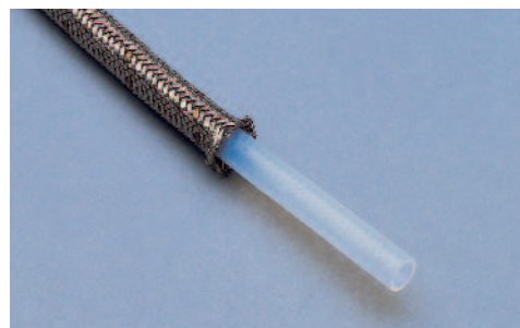
Each female SSPDS quick-connect coupling is attached to a PTFE hose encased in a flexible stainless steel outer braid to prevent hose damage and kinking during use.
