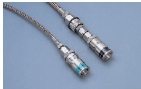
SSPDS hoses are available in 1/4" and 1/2" diameters. Honeywell Burdick & Jackson recommends including an in-line swivel (Catalog Number CA0311) when using the 1/2" hose to increase flexibility when aligning the quick-connect coupling key pattern.
