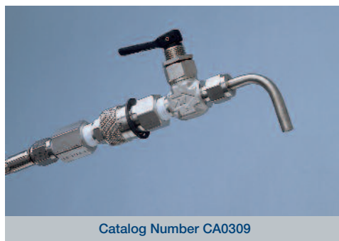
Each female SSPDS quick-connect coupling is attached to a PTFE hose encased in a flexible stainless steel outer braid to prevent hose damage and kinking during use.
