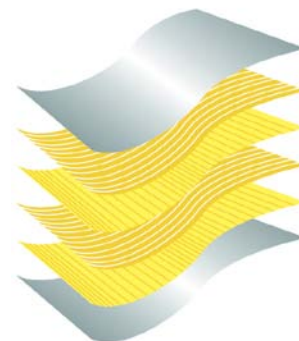
4 fiber and resin plies, consolidated with thermoplastic film to protect the composite package.
