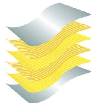
4 fiber and resin plies, consolidated with thermoplastic film to protect the composite package.
