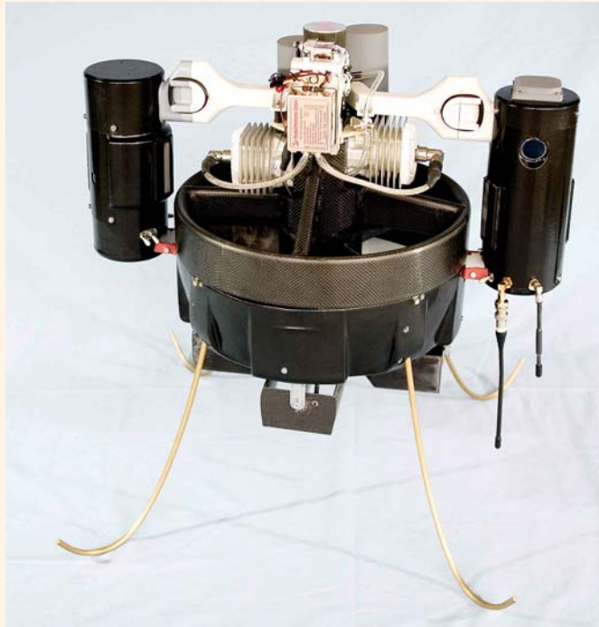
The ducted fan MAV has a 13 in. diameter shroud. Quick-change E/O and IR pods each contain forward looking and downward looking camera. (Honeywell)
