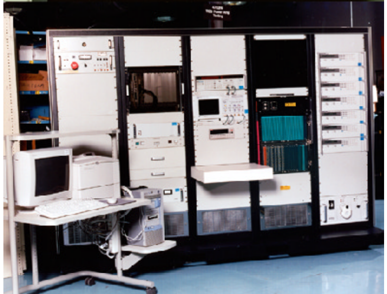
The fully modernized H3500 utilizes Pentium-based computer with Microsoft Windows NT operating system and a full array of commercial off-the-shelf "COTS" instruments.
