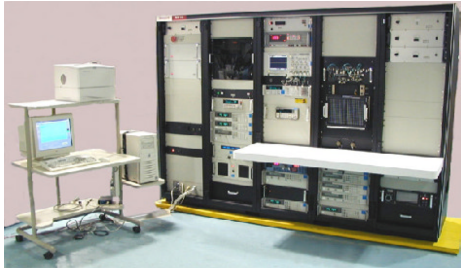
The fully modernized H2600 utilizes Pentium-based computer with Microsoft Windows NT operating system and a full array of commercial off-the-shelf "COTS" instruments.
