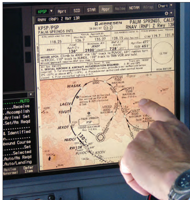
Honeywell G550 Capt Marc Lajeunesse points out the challenging terrain on the flightpath defined in the RNAV (RNP) Z Rwy 13R approach displayed on the copilot's MFD in the G550.
